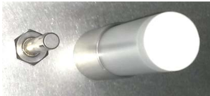
Figure 11: Plugged-in CO 2 sensor (right) and gas mixing head for CO 2
